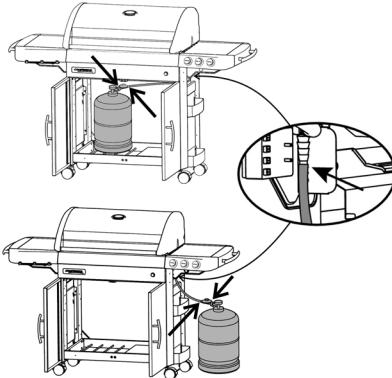
7)bubbles in the gas leak solution indicate that there are gas leaks.
